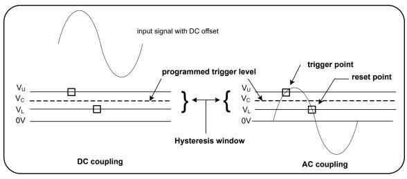
Figure 4-2 Using AC Coupling to Reach Trigger Points.
