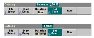
In terms of **Time**, the data logging duration is specified in hh.mm.ss format. The value is set using the rotary knob and arrow keys, or using the **[Shift]**ed numeric keys. By highlighting specific digits in the time window, greater resolution (i.e. minutes and seconds) of the logging time can be specified.
