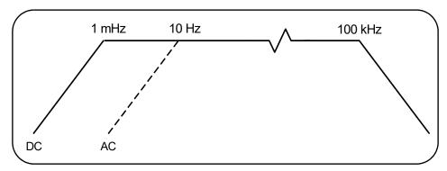
Figure 4-3 Measureable Frequency Range with Bandwidth Filter Enabled.
