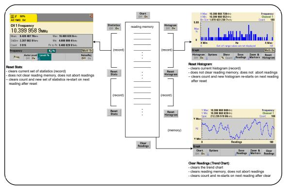
Figure 6-13 Reading Memory and Resetting/Clearing Graphics.
