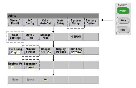
The format also applies to numeric readings within trend charts, histograms, limit testing, etc.
