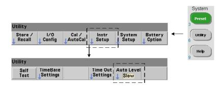
The minimum frequency at which auto-leveling can occur is set as shown.
