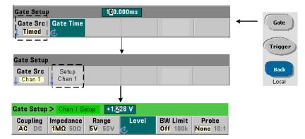
For external source **INPut[1]**, a **fixed** input threshold voltage must be specified in addition to the gate signal polarity. This is done using the command:
