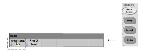
A frequency ratio measurement is the measurement of two signals in which one signal generally serves as a reference (Figure 3-2). The signals can be different wave shapes and applied to any 2-channel combination on the counter.
