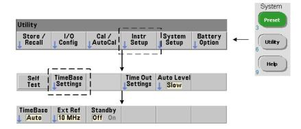
53210A measurements are based on a reference oscillator – also referred to as an internal/external clock or time base. A valid reference oscillator signal must be present for measurements to occur.
