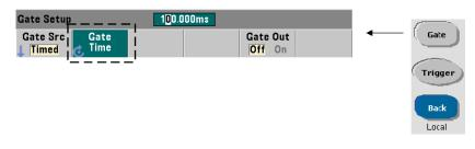
A measurement gate time can be specified directly with the command:
