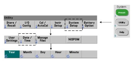
The date and time settings for the counter's real-time clock are set using the commands:
