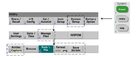
The content captured is the display state at the time the **[Utility]** key is pressed. The file format is selectable as either **bmp** (bitmap file format) or png (portable network graphics (bitmap) format). Files may be store in internal flash memory or to an external USB device.
