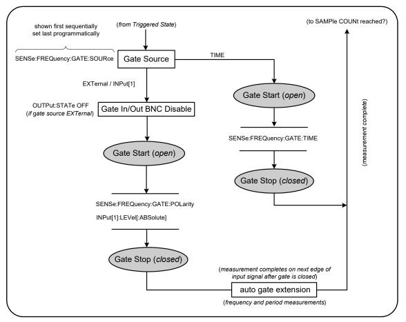
Figure 5-3 Trigger and Gate Cycle - Gating.
