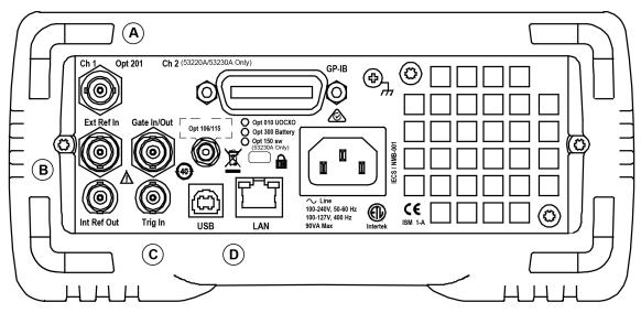
Figure 1-1 The 53210A Universal Frequency Counter/Timer.
