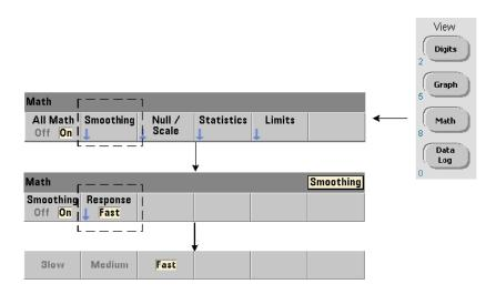
Measurements can be "smoothed" and scaled prior to performing math operations on the incoming data.
