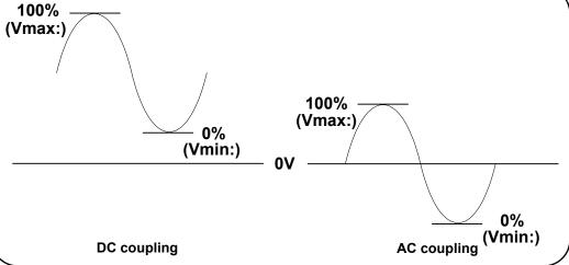
Figure 4-5 Input Coupling and Relative Threshold Levels.
