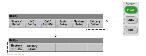
With Battery Option 300 installed and **enabled**, the 53210A counter can be operated using battery power for up to three hours.
