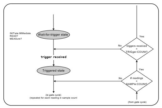
**Figure 5-4** The Counter 'Wait-for-trigger' State.
